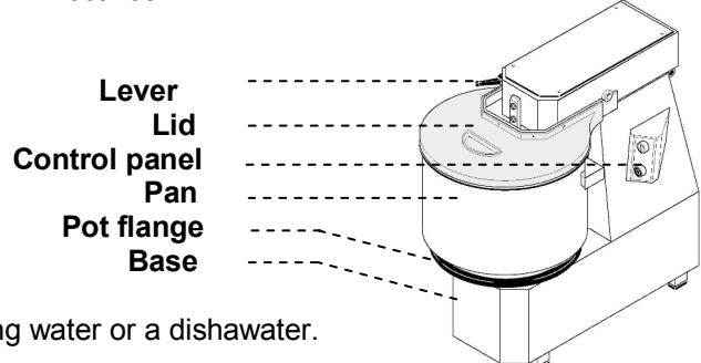
The bowl is removable to allow it to be washed in hot running water or a dishawater.
