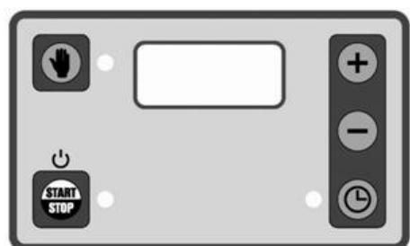
If you want to work without the timer, press the key with the “hand” symbol (manual) twice. The LED next to it will come on (it excludes the timer) and by pressing the “START/STOP” key the machine will start in manual mode.
