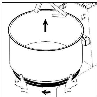
For removing the pan rotate the lower flange clockwise and lift the pan upwards (mod.CNS).
