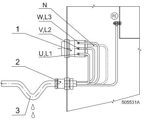
Figure 29 - Connection of main power inlet
