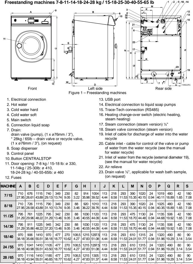
Table 4 – Freestanding machines, layout of machine components (dimensions stated in mm / inches)
