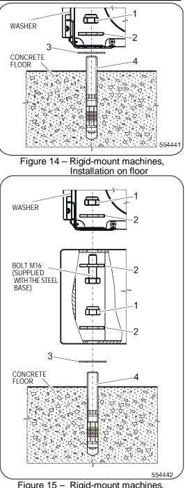
Figure 15 – Rigid-mount machines, Installation on a steel base and floor
