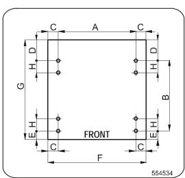
Figure 11 – Rigid-mount machines 18-24-28 kg / 40-55-65 lb – medium spin
