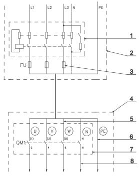
Figure 27 – Machine connection to electrical network (with a residual current device) <sup>505529</sup>
