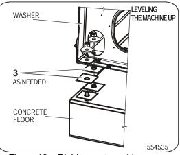
Figure 16 – Rigid-mount machines, 18-24-28 kg / 40-55-65 lb – medium spin
