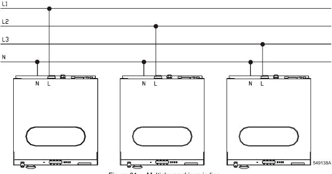
Figure 31 - Multiple machines in line
