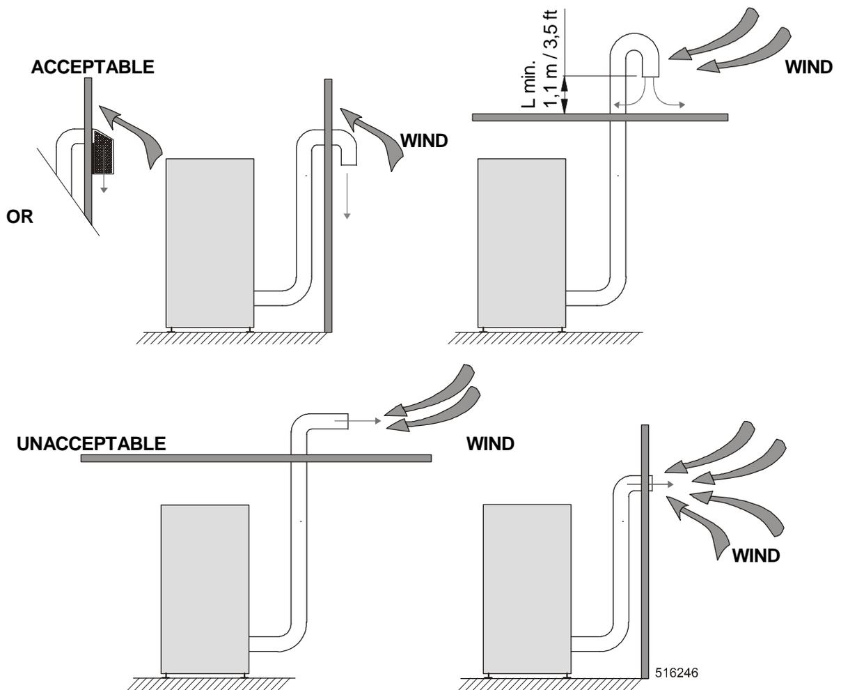
Fig.8.8.2.B. Individual exhaust duct
