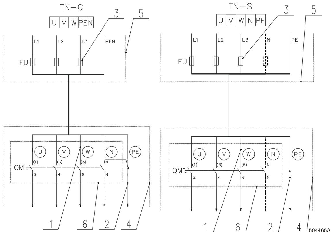
Fig.8.4 A. 3-phase machine connection to electrical network
