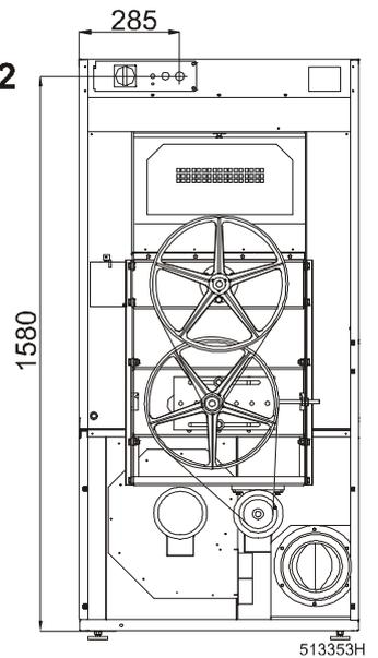
Fig.7.9. Dimensions and components of the machines 11kg (24lb), 13kg (27lb), 16kg (35lb)
