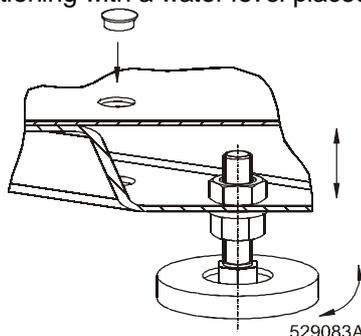
**LOCK LEVELLING LEGS WITH SAFETY NUTS INSTALLED IN ADVANCE.**
