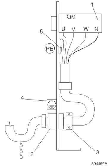
Fig.8.4.D. Main power supply connection
