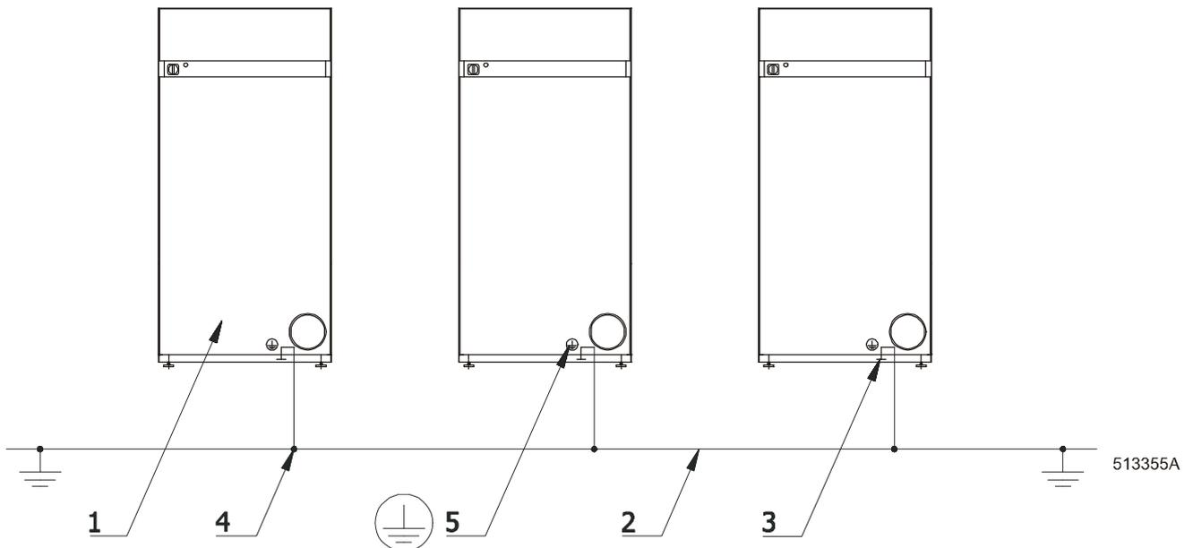
Fig.8.4.E. Protective machine connection
