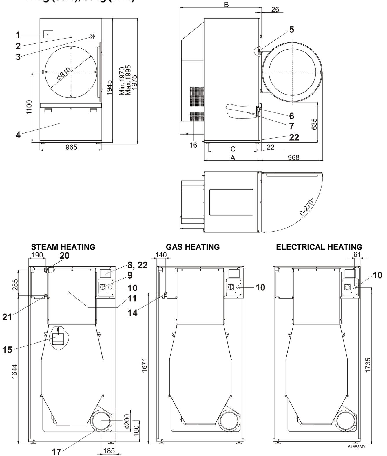
Fig.7.11. Dimensions and components of the machines 24kg (53lb), 35kg (77lb)
