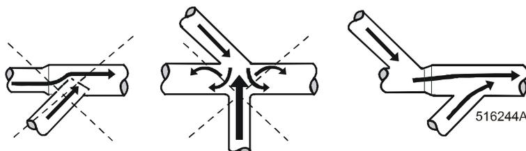
Fig.8.8.2.A. Pipe connections
