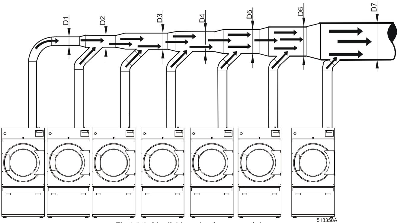
Fig.8.8.3. Manifold venting for range of dryers
