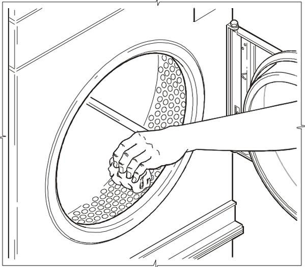
Fig.8.11. Inner drum cleaning
