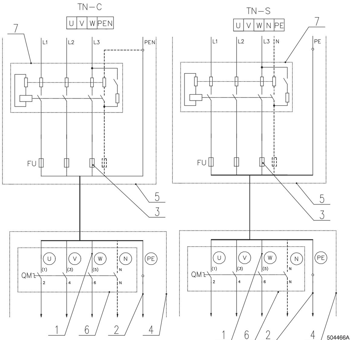
Fig.8.4.B. 3-phase machine connection to electrical network
