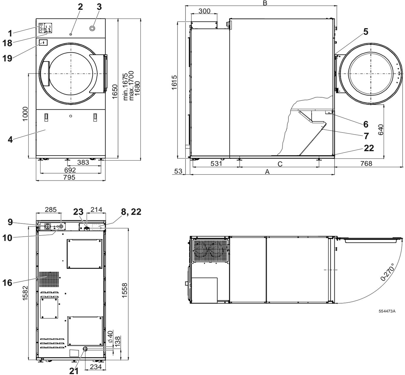
Fig.7.10. Dimensions and components of the machines 11kg (24lb) HP, 13kg (27lb) HP, 16kg (35lb) HP with heat pump
