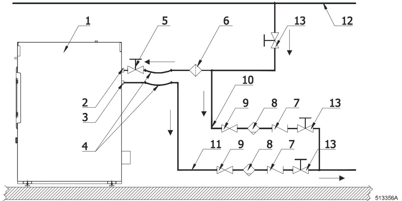
Fig.8.7. Scheme of steam lines
